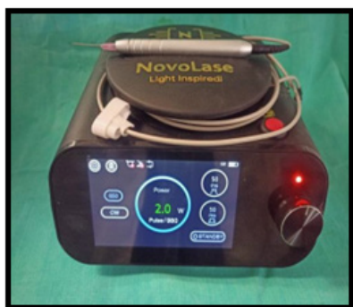
Figure 1: Diode laser: 980 wavelength, power-2 watt, continuous wave.
